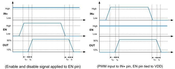
Figure 2. Enable and Disable Function Using EN Pin
